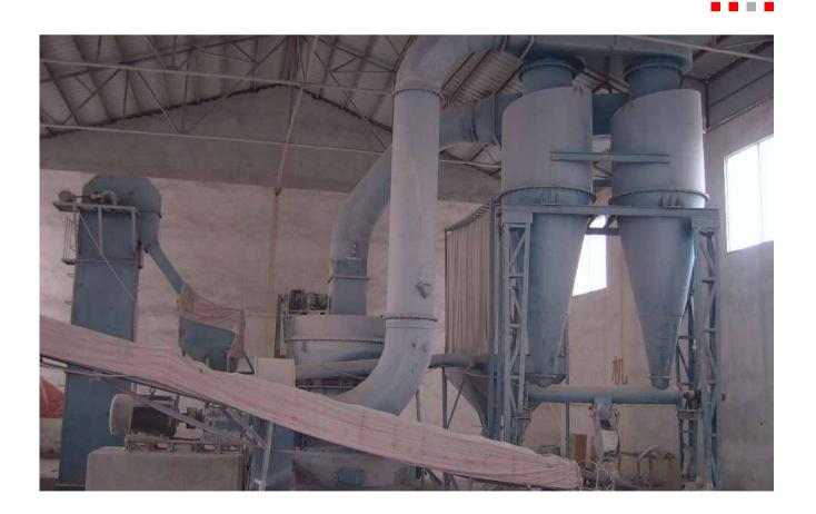
The diameters of each part of rollers and rings are different, the upper part is big and the lower part is small, then they formed a trapezium form. This form can reduce materials' sliding speed downwards and prolong the grinding time for materials, thus the grinding efficiency is increased.; the
