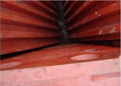
The equipment consists of bracket, jaw, eccentric shaft, jaw plate and toggle plate etc. Eccentric shaft is driven to rotate by motor and jaw runs on adjusted track to crush materials in crushing chamber. The bracket is welded by steel plate. On the front arm of bracket, jaw plate is fixed by wedge-shaped bolt. Edge protection plate is equipped on inside wall of bracket to prevent abrasion.
